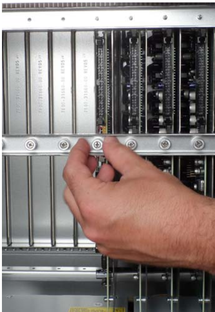
Figure 7. Securing a card to the Stage 64 chassis
