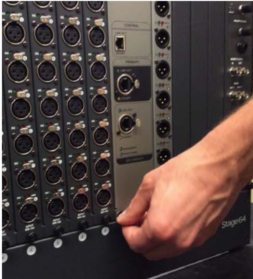
Figure 6. Tightening one of the four front captive thumbscrews
