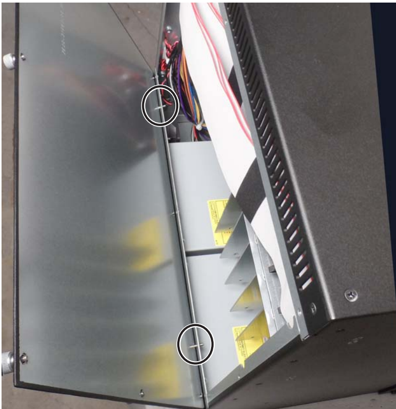
Figure 9. Back panel guide pins
