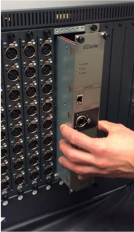
Figure 4. Sliding the card into the Stage 64
